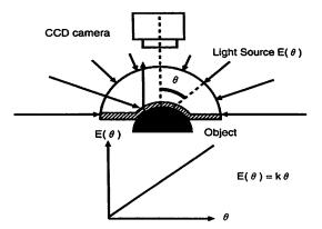
Figure 9. Function of Light Source in Axial Rotation.
