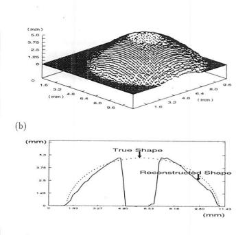
Figure 5. (a)Reconstruction of Spherical Object.(b)Cross Section of (a).
