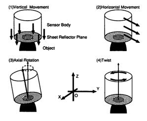
Figure 1. Four types of tactile sensor movement.
