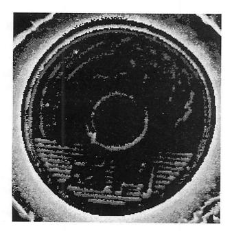
Figure 6. Reconstruction of 5 Yen Coin (22mm in Diameter).
