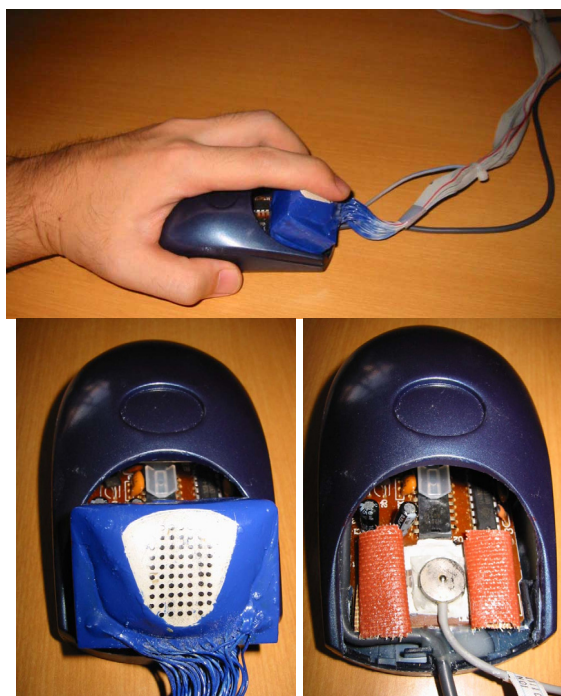
Fig. 20. Electric Mouse. 64electrodes, 2.0mm interval.(Top) Whole view (Bottom Left) Front view. (Bottom Right) Load cell to measure finger pressure.
