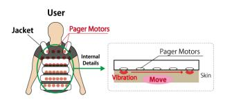
Figure 6 Overview of the stroking system
