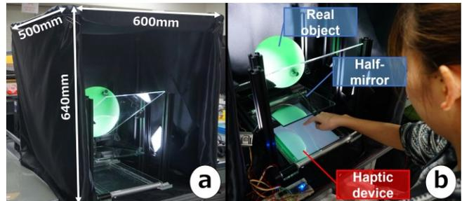
Figure 1. Prototype system.
