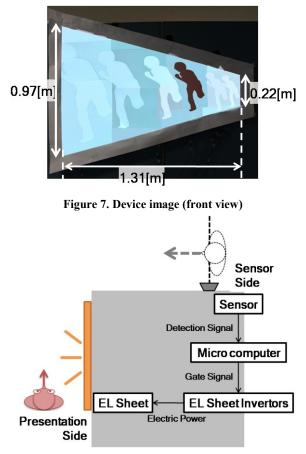
Figure 8. System diagram (top view)
