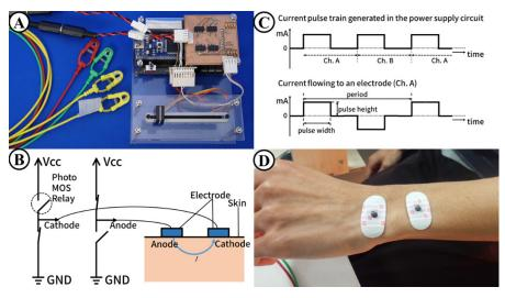
**Fig. 1.** (A) Electrical Stimulator. [2] (B) Two Photo MOS relays for one channel to allow a change of the channel state. (C) Monophasic current pulse train generated in the current control circuit is converted to biphasic pulses by switching the state. (D) Electrodes on dorsal part of the wrist.
