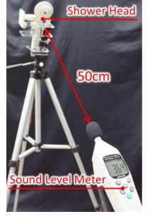
Figure 8 Setup to measure the sound level of operating volume: The sound level meter was located 50 cm away from the showerhead.
