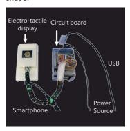
Figure 4. Overall view of the prototype.
