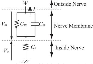
Figure 5 Simplified model of electrical nerve stimulation.
