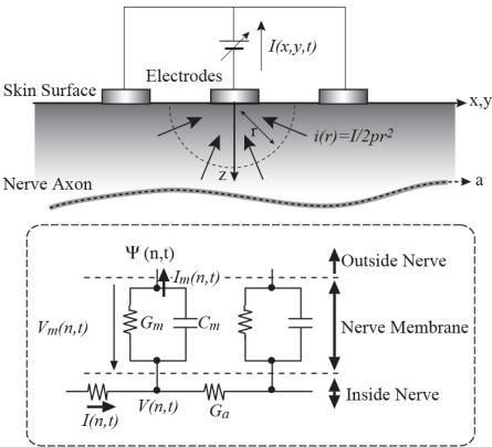
Figure 2 Electrical representation of electrical stimulation. Electrical current I from the skin surface generates a potential distribution. The potential distribution  $\Psi$  along the nerve axon generates membrane current  $I_m$ , resulting in a membrane voltage difference  $V_m$ .  $G_m$ : membrane conductance,  $C_m$ : membrane capacitance,  $G_a$ : internal conductance.
