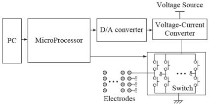
Figure 9 Typical system architecture of an electro-tactile display.
