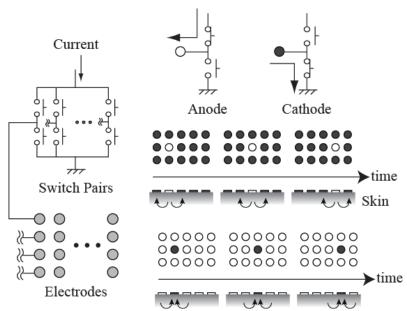
Figure 11 Scanning stimulation using a switching circuit. A pair of switches changes the state of electrodes between anode and cathode. The spatial pattern is obtained by temporal scanning.
