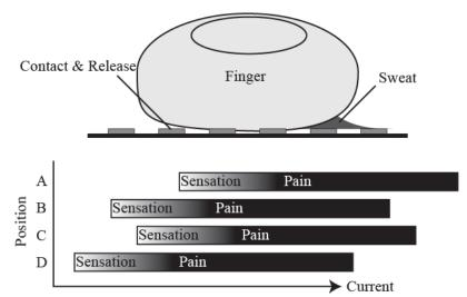
Figure 13 Two factors contributing to the sensation variability of electro-tactile displays. (Top) Temporal changes caused by sweat and contact. (Bottom) Spatial variation of thresholds.
