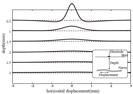
Figure 3 Activating function of cathodic current from a single electrode, assuming the nerve runs parallel to the skin surface.
