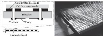
Figure 12 Electrode structure and conductive gel. The electrode surface is gold coated and the wiring is on the other side of the substrate. The conductive gel works as a diffuser.
