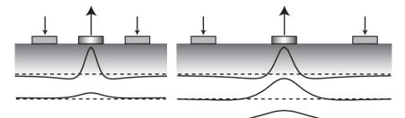
Figure 4 Relationship between the activating function and the diameter of the concentric electrode. A larger inter-electrode distance results in greater and deeper stimulation.
