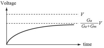
Figure 6 Step response of the membrane voltage difference
