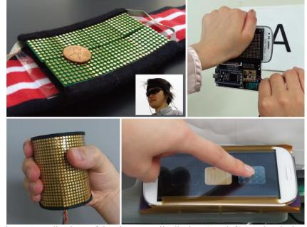
Figure 1 Applications of the electro-tactile display. (Top left) Forehead stimulation for a tactile–vision substitution system (TVSS) [1]. (Top right) TVSS of palm type [4]. (Bottom left) Cylindrical type for virtual-reality application [5]. (Bottom right) Touch-panel type using transparent electrodes [6].
