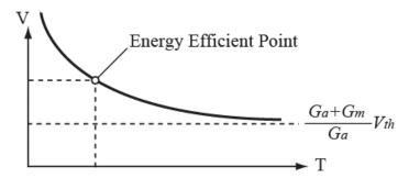
Figure 7 Strength–duration curve showing the relationship between the pulse width and pulse height when the nerve is only just stimulated.
