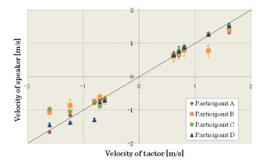
Fig. 3. Subjectively equivalent velocity.
