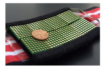
Fig. 8 512 (32 × 16) electrodes module for the forehead.
