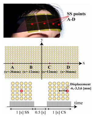
Fig. 9 Two point discrimination test setup.
