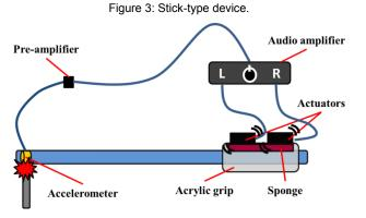
Figure 4: System configuration.
