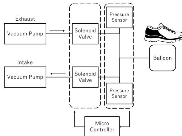
**Fig. 3 System configuration of pneumatic balloon shoes**
