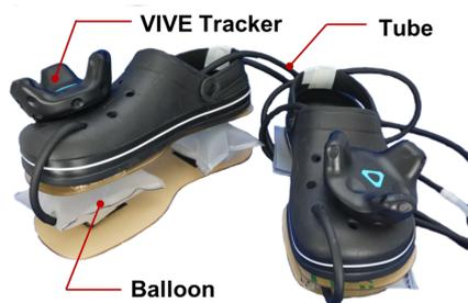
**Fig. 1** Height presenting shoes using pneumatic balloons
