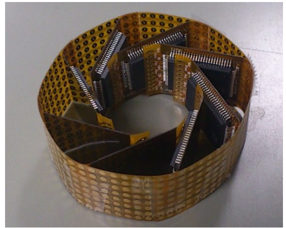
Fig. 3 Cylindrical shape by connecting flexible electrode units.
