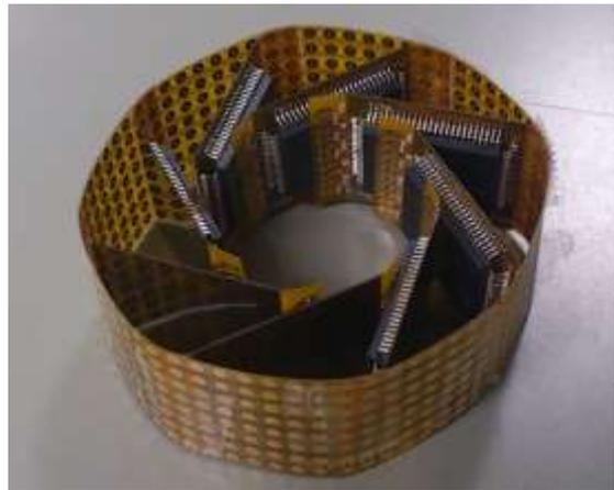
Fig. 3 Cylindrical shape by connecting flexible electrode units.
