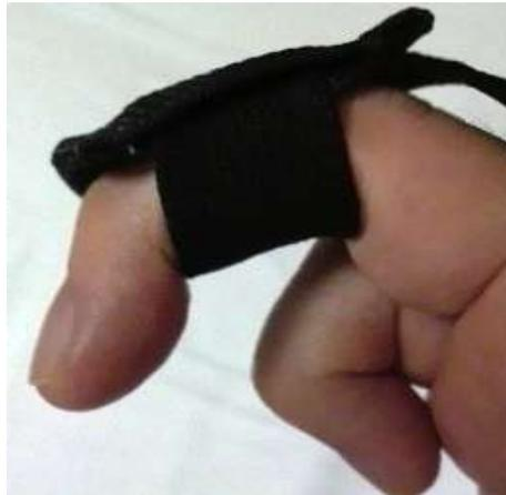
Fig. 5 Wrap-type electrocutaneous display hinders bending of the finger.
