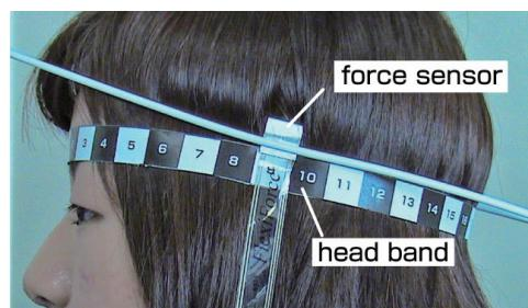
Fig. 2 Pressure distribution measurement for the hanger reflex.
