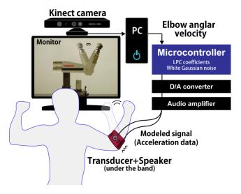
**Figure 6.** Hardware setup of the prototype system. In AR Jointonation system, we will use an HMD instead of the monitor to superimpose virtual robot arms on the user's arms.
