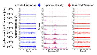
**Figure 5.** *Recorded vibration (left), example of LPC-modeled vibration (right), and overlaid spectral density (center).*
