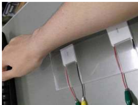
Fig.1 Two peltier elements to give heat to the skin
