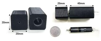
Figure 2 Size of the device
