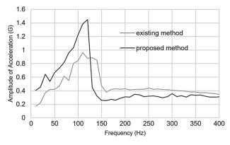
Figure 5 Frequency response of each vibrotactile actuator
