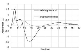
Figure 4 Time response of each vibrotactile actuator
