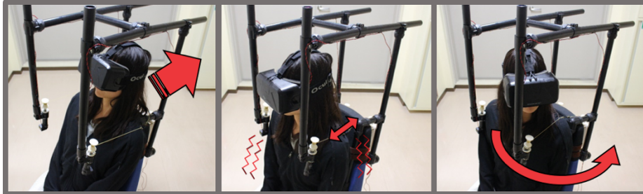
Fig. 4. Sensation induced by HapPull (left: pressure; center: vibration; right: torque)
