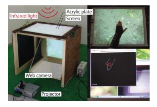
Fig. 8 Position sensing and image output
