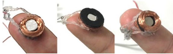
Figure 3: Appearance of the transducers (left: Type I, middle: Type II, right: Type III)
