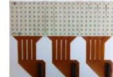
Figure 2. Picture of the electrode array used. The inter-electrode distance is 10 mm. The electrodes are arranged in a 8x24 grid. Electrode numbering starts at the lower left corner and works columnwise.
