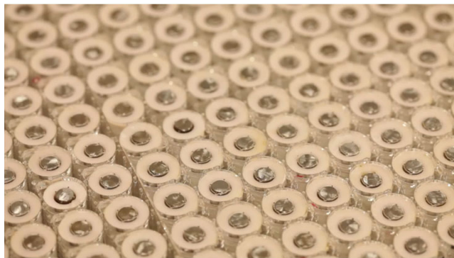
(UIST2011) FingerFlux: Near-surface Haptic Feedback on Tabletops, Weiss, Wacharamanotham, Voelker, Borchers. https://www.youtube.com/watch?v=trM7mXOjNFY タブレットの下に電磁石、指に磁石を取り付ける
