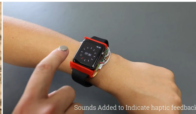
(CHI2019) Magnetips: Combining Fingertip Tracking and Haptic Feedback for Around-Device Interaction Jess McIntosh, Paul Strohmeier, Jarrod Knibbe, Sebastian Boring, Kasper Hornbæk https://www.youtube.com/watch?v=-IBZ2xzx2jU スマートウォッチの下の電磁石、指に磁石。磁石は位置検出にも用いる
