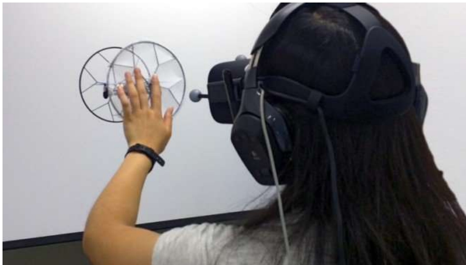
https://dl.acm.org/doi/abs/10.1145/3282894.3282898 (MUM2018) VRHapticDrones: Providing Haptics in Virtual Reality through Quadcopters, Hoppe et al.
