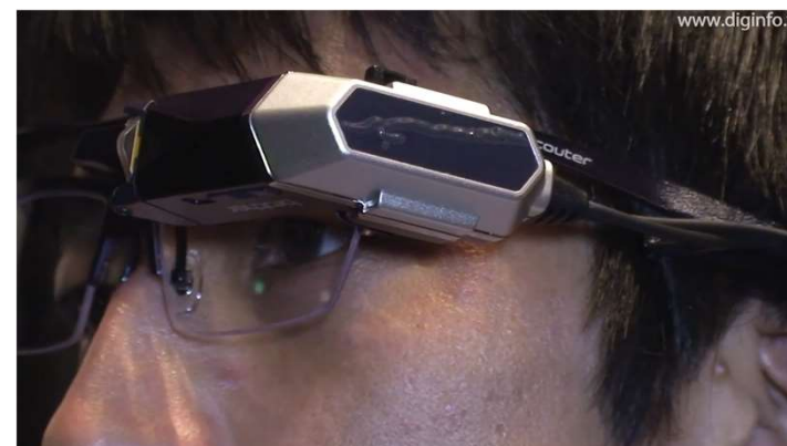
Head-mounted display projects directly onto the retina : DigInfo https://www.youtube.com/watch?v=9I0hF0cbw8E
