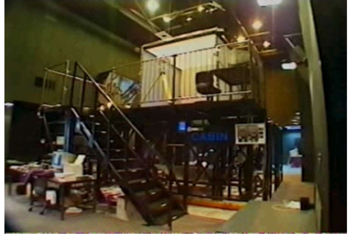
LCD shutter type IPT system: CABIN @ U-Tokyo
