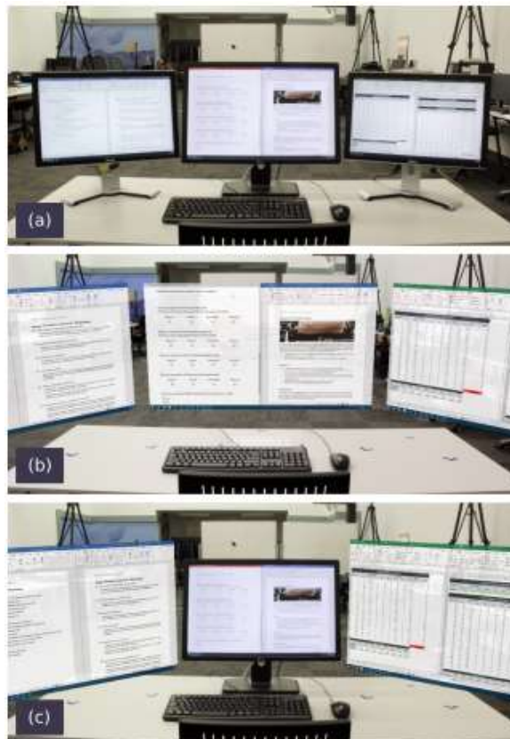
Figure 2: (a) Physical condition had three monitors side-by-side; (b) Virtual condition had three monitors rendered through HoloLens; (c) Hybrid condition combined a central physical monitor with two peripheral virtual monitors.
