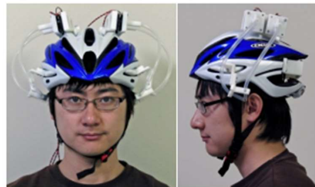
Kojima et al: A Novel Wearable Device to Present Localized Sensation of Wind(2009) https://dl.acm.org/doi/10.1145/1690388.1690399 スピーカーを使った高速応答の風提示を「耳」に対して
