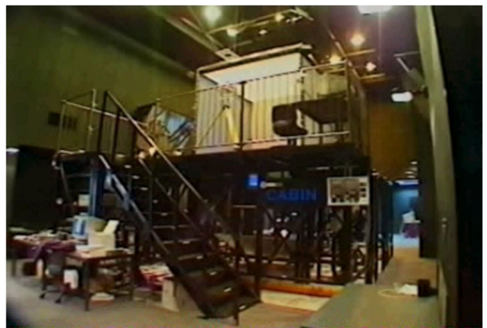
LCD shutter type IPT system: CABIN @ U-Tokyo
