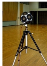
Put Point source speaker on the stage.
