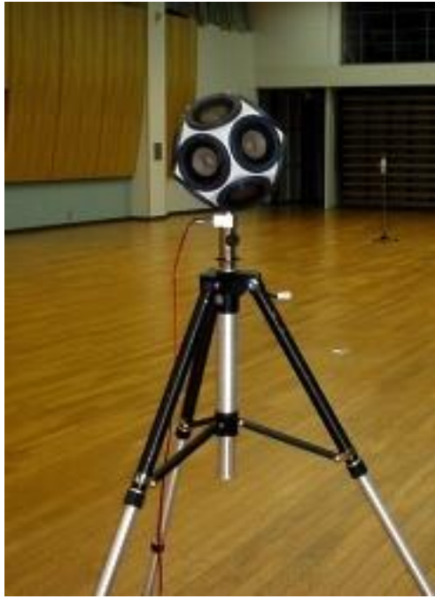
Put Point source speaker on the stage.
