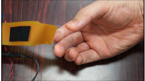
64 transparent electrodes are made of ITO (Indium, Tin, Oxide)
