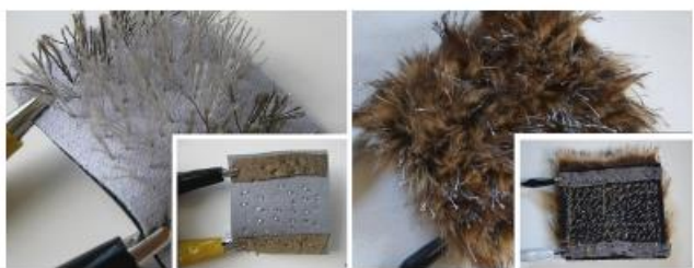
Figure 3: Perner-Wilson and Satomi's conductive thread stroke sensor (left) [12], our conductive fur touch and gesture sensor (right).
