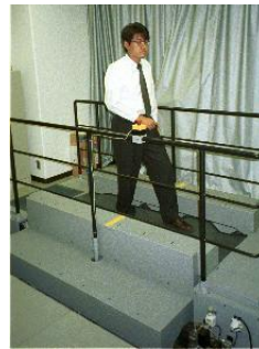
ATR GSS (ground surface simulator)
