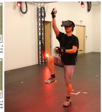
Figure 1: Users climb up with March-and-Reach by grabbing a virtual rung with two buttons, and then raising and lowering a foot to virtually step up on the next rung. The transparent red shapes represent the user's virtual hands and feet.
