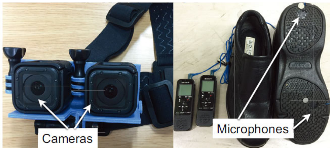
Figure 1: (Left) Stereo cameras, (Right) Microphones to capture foot strikes.
