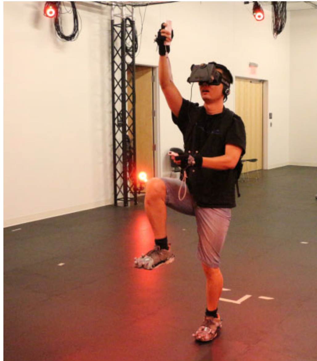
Figure 1: Users climb up with March-and-Reach by grabbing a virtual rung with two buttons, and then raising and lowering a foot to virtually step up on the next rung. The transparent red shapes represent the user's virtual hands and feet.
