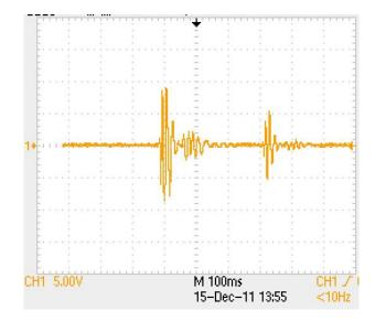
Figure 2. Actual output voltage from the audio speaker
