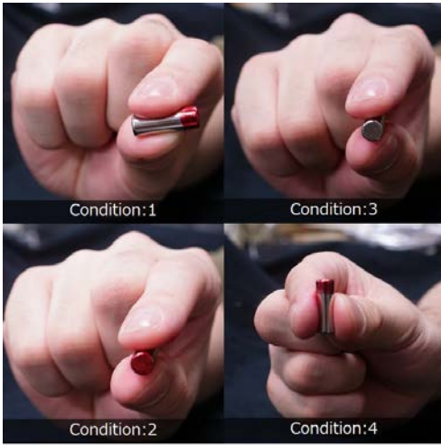
Fig. 3 Orientation of the magnet (N pole at the red end). In all cases, the hand faces the front of the coil, as shown in Fig. 5
