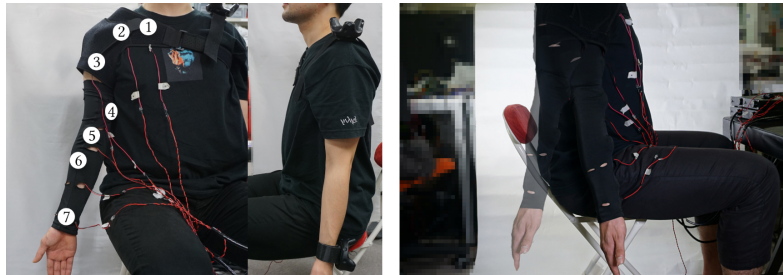
Figure 1: Left: positions of vibrators and trackers. Right: an image of the induced kinesthetic illusion.
