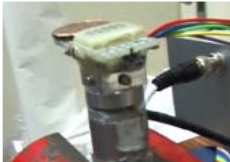
Figure 5 Force based current control. Force sensor with 6DOF is located under 2x5 electrode array.
