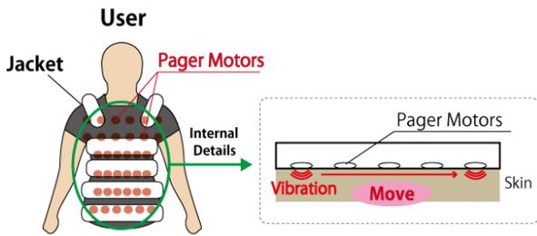
Figure 6 Overview of the stroking system
