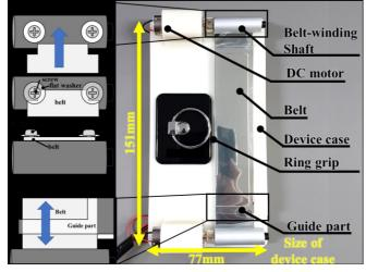
Figure 2. Configuration of the prototype
