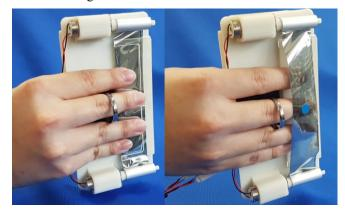
Figure 1. Overview of the protptype. (Left) Vibration is transmitted to the fingertip by touching on the belt in "On belt condition", and (Right) to instep of the fingers by covering fingers in "Under belt condition"
