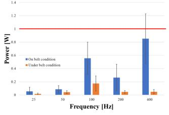
Figure 3. Answered power in "on belt condition" and "under belt condition" compared with the vibrator driven at 1W. Red line shows the electric power applied to the comparative device.
