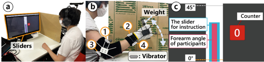
Fig. 1. (a) An overview of the environment as for experiment 1. (b) Positions of the vibrators and the markers. (c) Screen display of the sliders for movement control.
