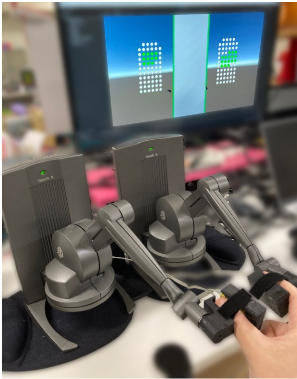
Fig. 2. Force and electro-tactile rendering; the 64 electrodes attached to each of the two devices, the green circle represents the electrode that is in contact with the edge of the presented object (in the center of the monitor), and the corresponding electrode is being stimulated.
