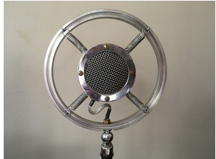
Crystal microphone or piezo microphone
