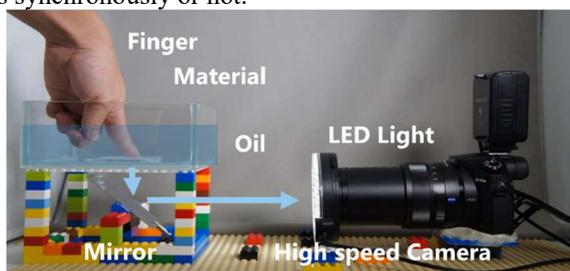
Fig. 1. Measurement System[1]
