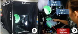
Figure 1. Prototype system. (a) Overall view. (b) Inside view.
