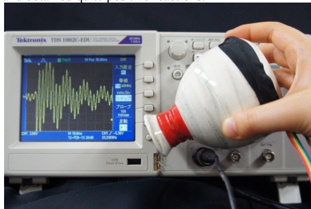
Fig. 3. Sake-bottle-shaped device with a vibro-tactile actuator
