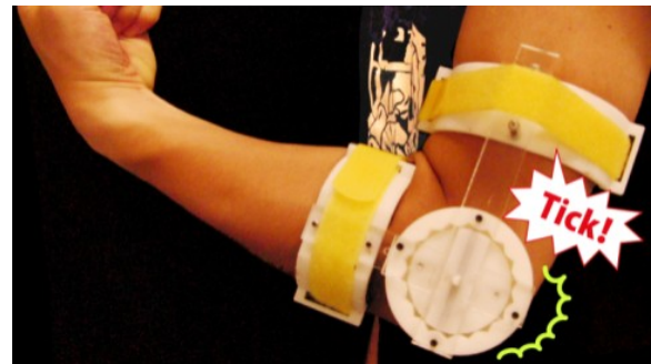
Figure 1. Rotary switch feeling feedback at the elbow
