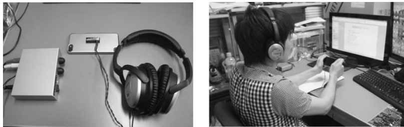
Fig. 1. Left: The main components of the apparatus, consisting of headphones, an amplifier, and the vibrating device. Right: Overview of the experiment.
