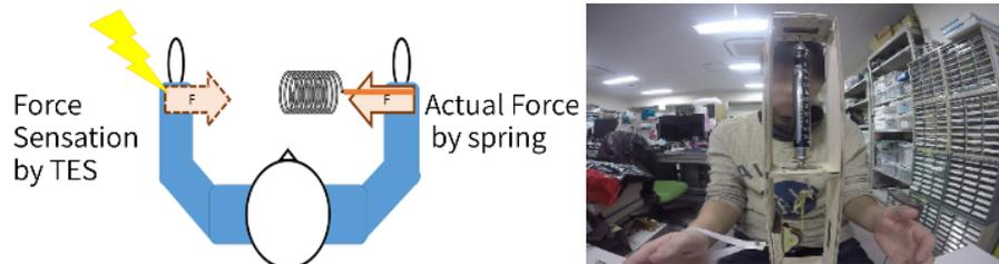
**Fig. 2.** Measurement of perceived force sensation. (Left) Concept image. (Right) Actual system
